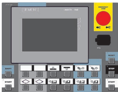
CONTROL PANEL: SIEMENS (X-CNC)
